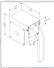
The Abanaki TubeTastic! oil skimmer can be used on machining centers with little or no access to the coolant sump from above. This unit can skim oil from chip conveyors or even totally enclosed machining centers!
