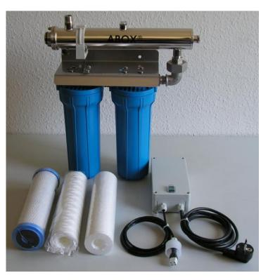
Save disinfection by UV light requires that the treated water has a good UV transparency and is free of particles and turbidity. This is achieved by prefiltration. The compact type unit ABOX<sup>®</sup>WAS combines the prefiltration and the UV disinfection in a common device. The compact and space saving design is making it ideal for using on boats, in holiday houses or shelters or for mobile applications.
